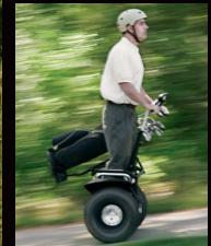
Segway Smart Motion<sup>™</sup> technology consists of an intelligent network of sensors, mechanical assemblies, and control systems that enable the Segway PT to balance and move on two wheels. The second you step on, five micro-machined gyroscopes and two accelerometers sense the changing terrain and your body position at 100 times per second – faster than your brain can think.
